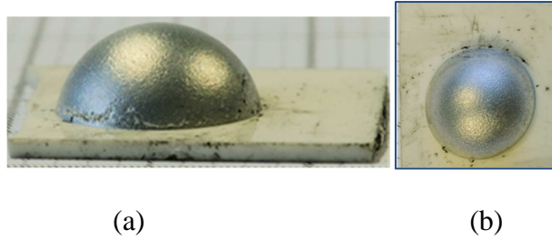
Figure 5. Lateral (a) and top (b) views of the AlSiMg drop solidified on the \text{Al}_2\text{O}_3 substrate after the wetting test under vacuum.
