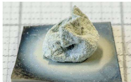
Figure 10. Image of the SLMed AlSiMg sample solidified on \text{Al}_2\text{O}_3 substrate, after the wetting test performed under Ar- atmosphere.
