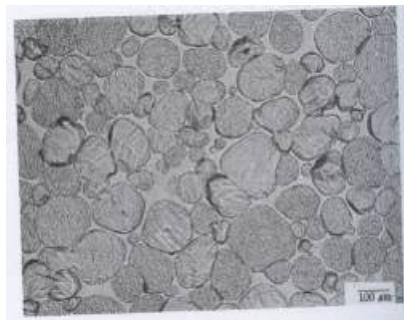
Fig. 8. Typical microstructure of a LPS system with the phase diagram characteristics shown in Fig. 6 [60].
