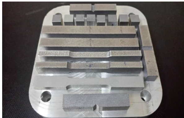
FIGURE 4. The arrangement of samples on the SLM platform
